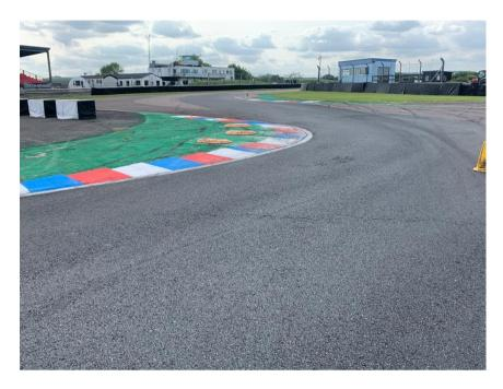
The kerb and the white line can be used, but no part of the tyre contact patch can be on the green or the sausage kerbs.
